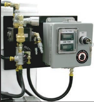
Keep track of the time spent on a job and total hours on your abrasive blaster. Know your cost, control your cost & set up a preventative maintenance program for your blast equipment.
